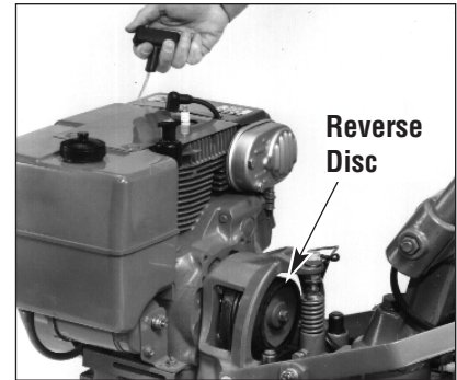
Figure 5-25: Checking Reverse Disc in NEUTRAL.
